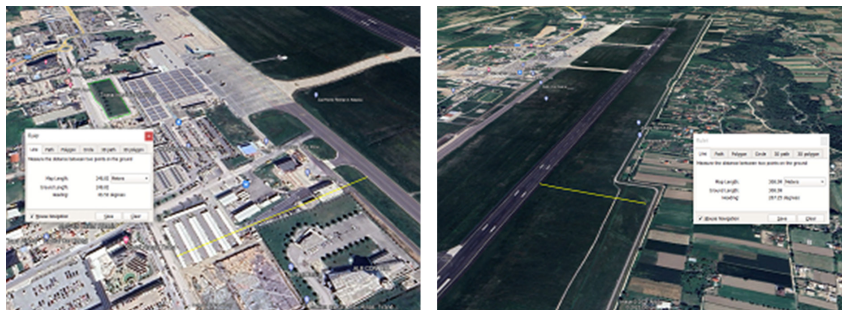
Figure 7. Distance between two proposed FATO-s and taxiways and runways
